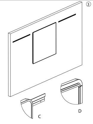
Draw a level line the total length of the linked boards 2 1/8" below of the deisred finished height of the boards
