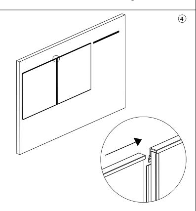
Hang left side board onto bracket and slide into middle board. Repeat with right side board. Double-sided tape on the back in bottom corners ensures complete stability.
